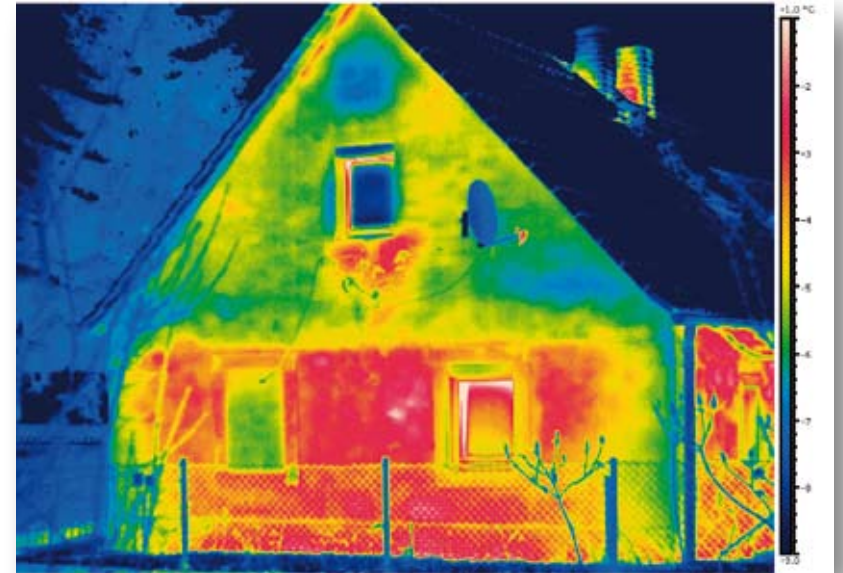
Image taken with 640x480 pixel resolution and <45mK thermal sensitivity. The increased number of pixels will result in a much clearer picture where small details are very visible.
