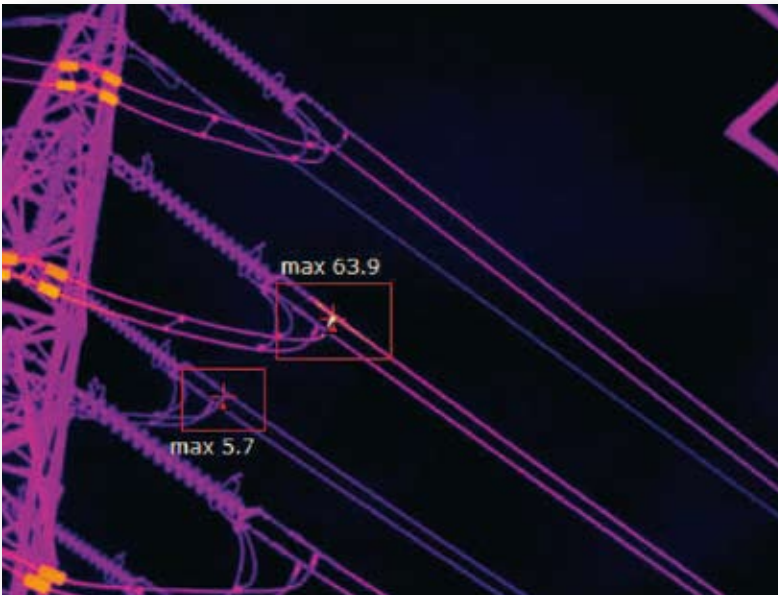
Image taken with 640x480 pixel resolution and <45mK thermal sensitivity. Notice how the hot spot now is clearly visible and that the increased number of pixels will result in an even more accurate temperature reading in the hot spot. It is now clear that there is a problem in the power line.
