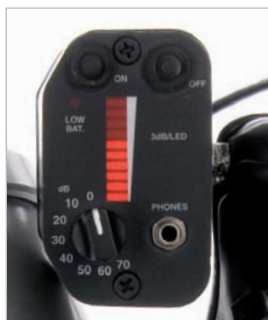
LED display and sensitivity dial
